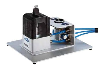
Hektor separates milled PCBs carefully and fast. The off-cut material is removed smoothly and precisely. The matrix consists of two parts. This ensures easy and cost-saving change of the blades. Compressed air is used for the separation process. The operating pressure can be set on the machine. When the foot switch is pressed, the off-cut is punched out. The off-cuts are collected in the collecting box. When the gate is opened the waste material can be extracted.
