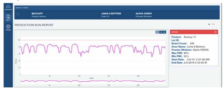
The Vantage system can connect with automated systems on your ovens AND shares data with other factory systems, such as MES. Production data and analytics are provided to MES for the best in automated process control and traceability.
