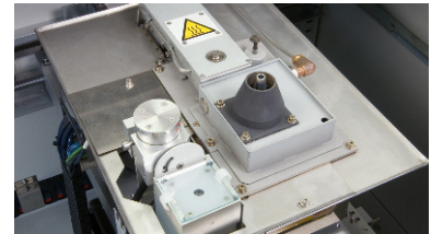
SOLDER BATH AND PUMP ASSEMBLY WITH DROP-JET FLUX HEAD AND PROGRAMMING CAMERA
