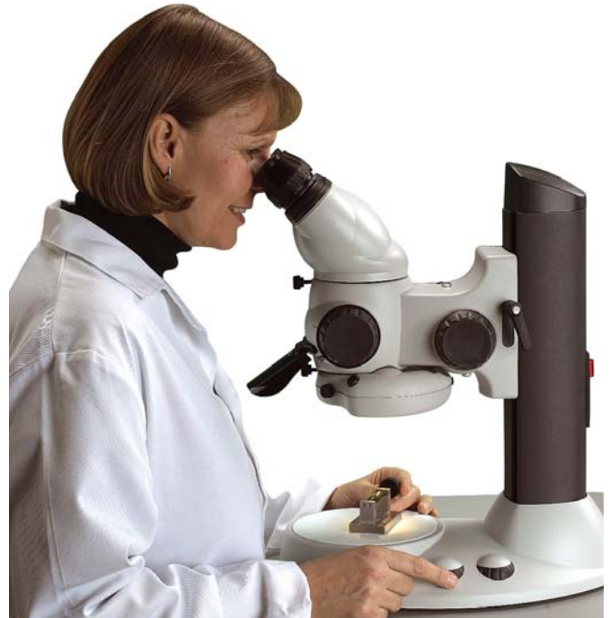
Beta bench stand with integral substage illumination.
