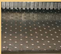
Low Mass Forced Convection Preheat Module
